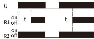
DPDT (One Inst.One Delay Output) 一瞬一延
